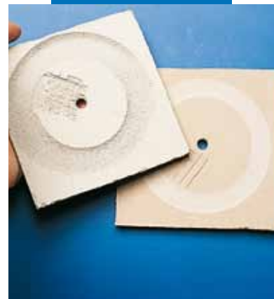
Taber abrasion executed on Ultraplan (right specimen) and on conventional levelling (left specimen) after 200 cycles
